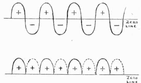
Fig. 5. Current from Rectifier
